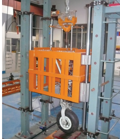
Fig. 7. Landing gear experiment platform
